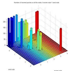
The above graph shows the total number of packets received by destination node during the simulation.
