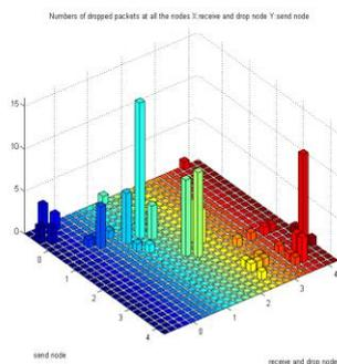
The above graph shows the number of packets dropped at all the nodes. The reason for packet drop may arise due to congestion, faulty hardware and queue overflow etc.
