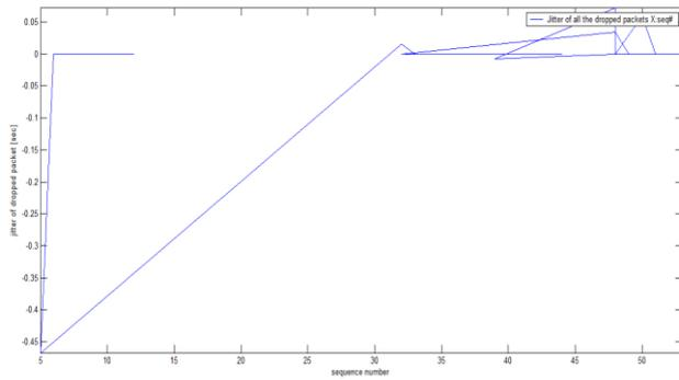
The above graph shows the jitter of all dropped packets. It is defined as the mean deviation of the packets from source to destination for number of vehicles.
