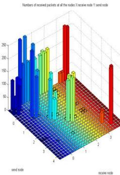
The above graph shows the number of packets delivered at all the nodes. Number of received packets refer to the number of delivered data packet to the destination.
