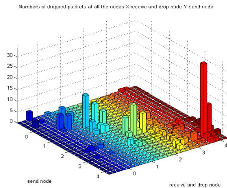
The above graph shows the number of packets dropped at all the nodes. Packet loss is measured as a percentage of packets lost with respect to packets sent.
