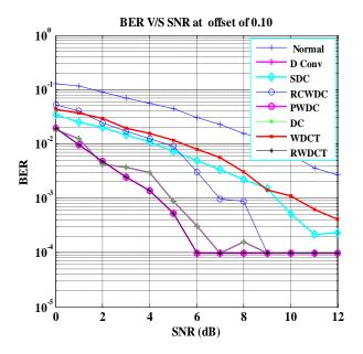
Fig. 4 BER v/s SNR for system with 0.1 offset
