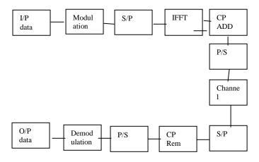
Fig. 1 OFDM Transceiver
