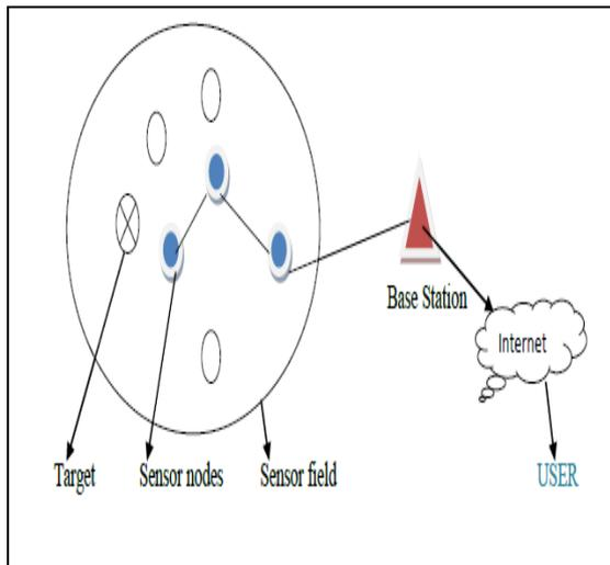
Fig.1. Architecture of wireless sensor network
