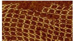
FIGURE 1. A DNA scaffolding for nanoelectronic circuits 100 nm
