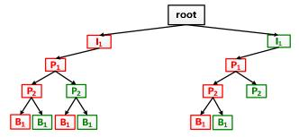
Fig. 6 Example of a QoET tree where packet  $P_1$  is expired and the available capacity of the connection is overcome with the transmission of  $I_1$  and  $P_2$  frames
