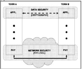
Figure 1: Based on the OSI model, data security and network security have a different security function [2].
