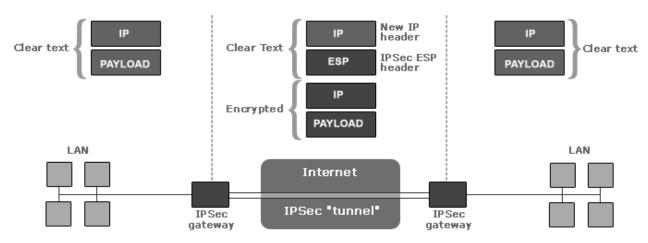
Figure 2: IPsec contains a gateway and a tunnel in order to secure communications.[17]
