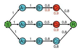
Fig. 2. Metric manipulation attack during the propagation of the flood packet from the source S to receiver R. A label above a link is the link's real SPP metric; a label below a link a node is the accumulated route metric advertised by the node.
