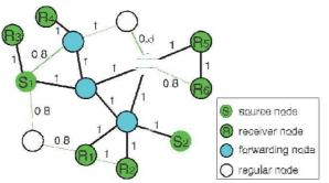
Fig. 1. An example of ODMRP-HT mesh creation for a multicast group with two sources (S1; S2) and six receivers (R1.R6); R6). The label on each link represents the value of the link's SPP metric.
